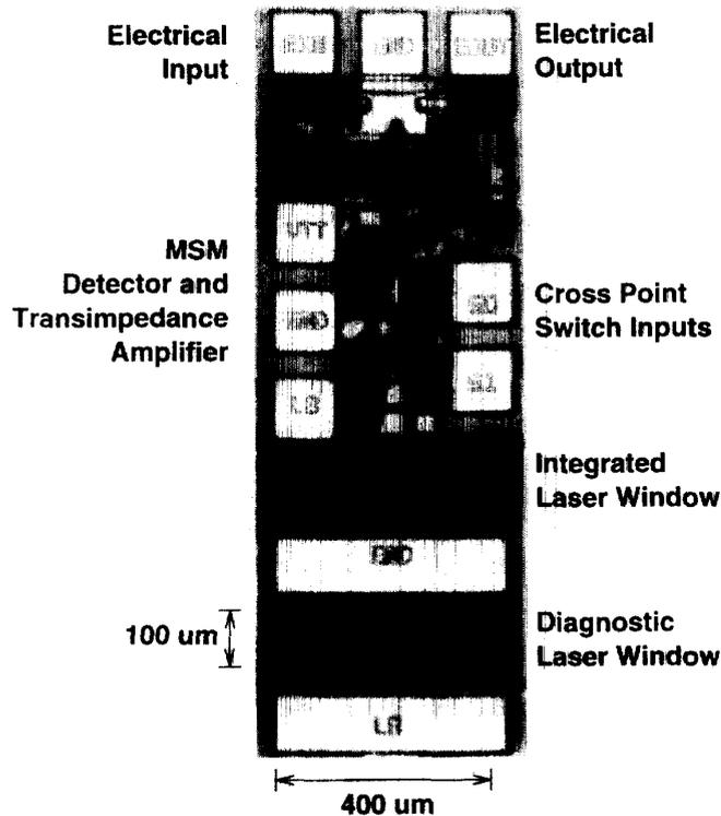
Figure 2: Electronic portion of OE-transceiver as received from foundry consisting of VLSI GaAs MESFETs (top) and windows exposing substrate (bottom). Each OE transceiver is approximately  $0.4 \text{ mm}^2$ .
