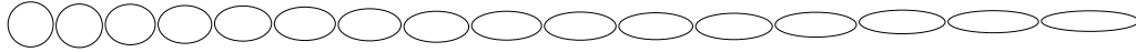
FIGURE 14. Extension of a solid placed in an initially Taylor-Green vortex (non-conservative formulation).
