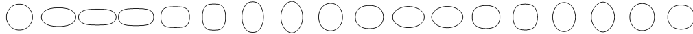
FIGURE 15. Oscillation of a solid placed in an initially Taylor-Green vortex (conservative formulation).
