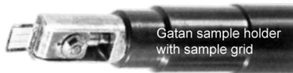
Figure 1: Close-up view of the Gatan 630 ultra high tilt holder with specimen grid.
