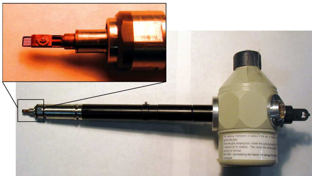
Figure 2.5: View of the Gatan cryo sample holder. The dewar can be filled with liquid nitrogen to cool the sample. The small image shows a close-up of the tip of the holder, where a high-tilt copper grid is inserted. The grid can be retracted between two copper plates to protect cryo specimens during transfer into the vacuum chamber.
