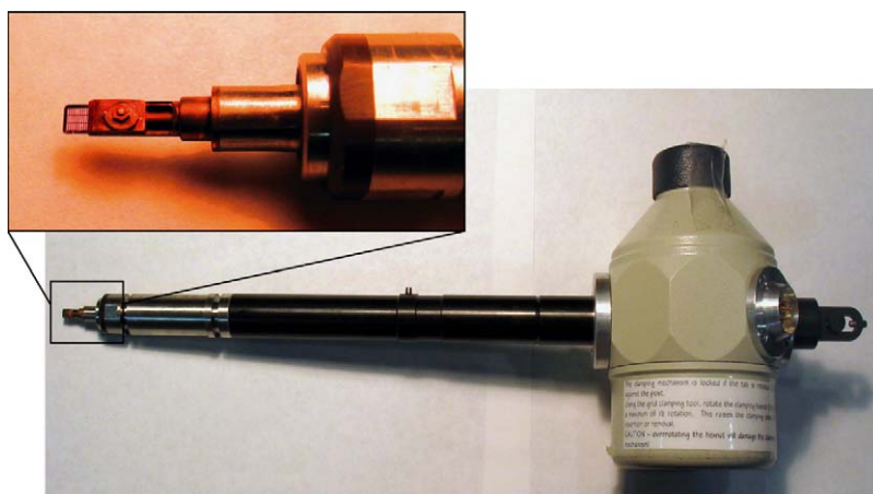
Fig. 4. View of the Gatan 630 high-tilt cryo sample holder. The dewar can be filled with liquid nitrogen to cool the sample; the specimen region is cooled by thermal conduction through a copper rod connecting it to this dewar. The small image shows a close-up of the tip of the holder, where a high-tilt copper grid is inserted. The grid can be retracted between two copper plates to protect cryo specimens during transfer into the vacuum chamber, and then extended so that it can be viewed at very high tilt angles (up to about \pm 80^\circ ).
