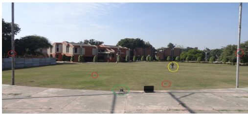
Fig. 6. Experimental deployment showing mobile anchor node, static sensor nodes, routers and gateway
