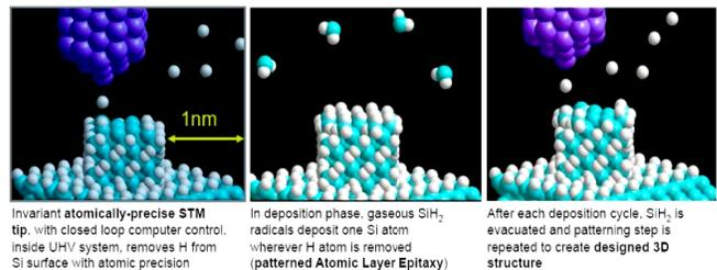
**Figure 1. Systematic removal of H from Si surface shows the concept of manipulating single atom [2].**
