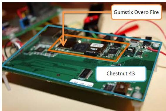
**Figure 4. Receiver (a): Gumstix Overo Fire module on a Chestnut 43 Daughterboard.**
