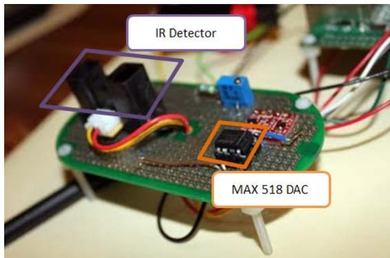
**Figure 5. Receiver (b): Daughterboard expansion to host additional DAC and IR detector for demo purpose.**
