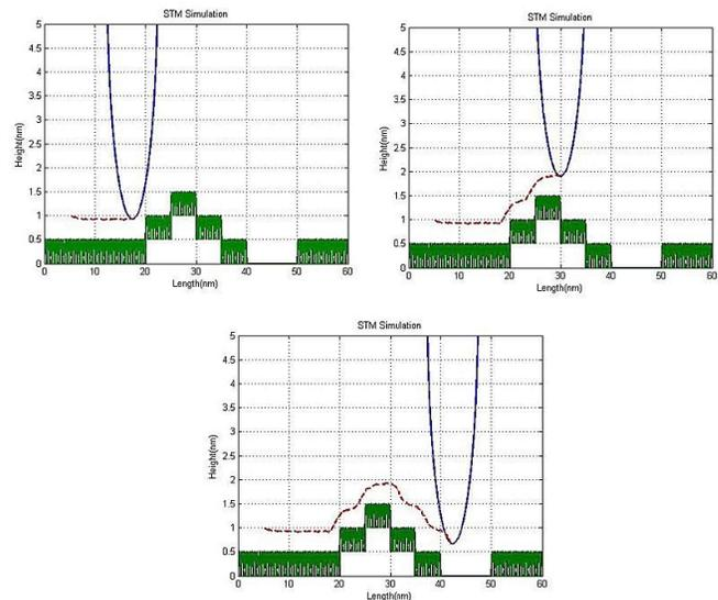
**Figure 6. Simulation results for real-time scanning of simulated randomized atomic surface.**
