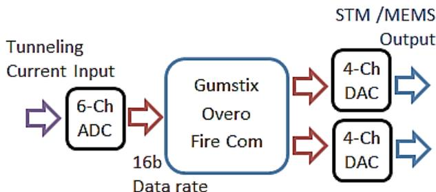
Figure 8. Upgraded system structure with high speed ADCs and DACs
