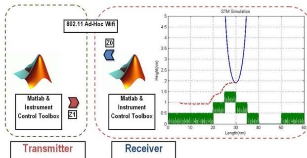
Figure 2. MATLAB simulation for controlling a STM tip through 802.11.
