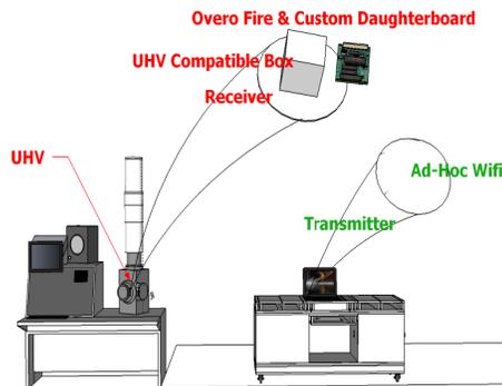
Figure 3. Hardware overview of the complete system.
