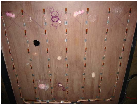
Figure 1. Composite panel with sensors
