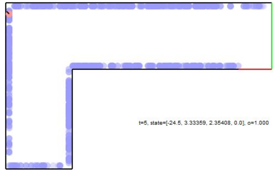
Figure 2: The same simulation after 5 time steps. Notice the belief state is much smaller due to the Roomba having hit a wall
