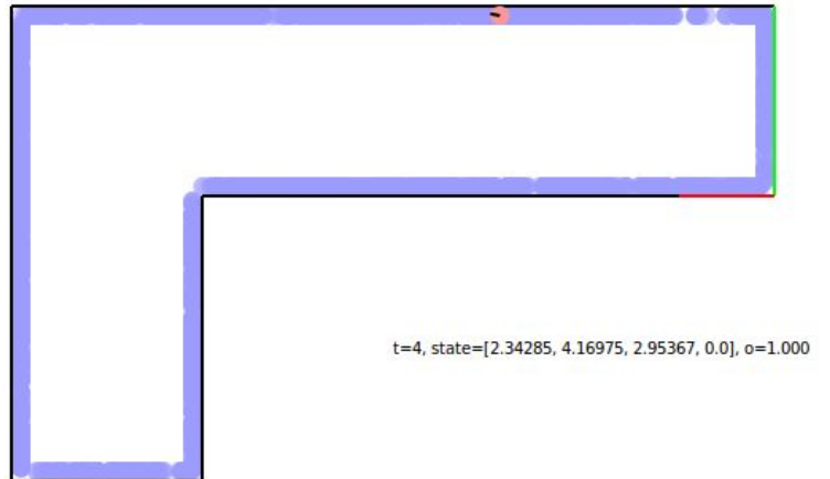
Figure 2: When the bumper sensor is used, the particle filter localizes to points along the wall when contact is made.
