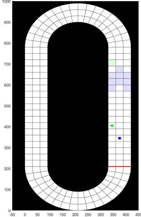
Fig. 1. Snapshot of track in state [5 2 7] where ego vehicle is in blue and other vehicle is in green. Possible actions for ego vehicle are highlighted in light blue and next position of other vehicle highlighted in light green for reference.
