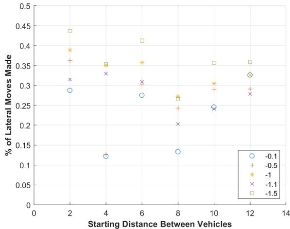
Fig. 4. Simulation Data: Lateral moves per action taken by the ego vehicle in pursuit of closing the gap between itself and the other vehicle before passing.
