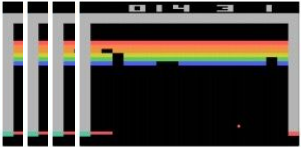
Current state s_t : 84x84x4 stack of last 4 frames (after RGB->grayscale conversion, downsampling, and cropping)
