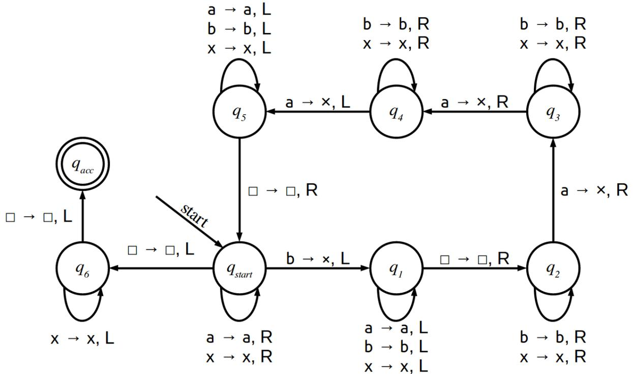
Here,  $q_{start}$  is the start state, and  $q_{acc}$  is the accepting state. As usual, we assume that all missing transitions implicitly cause  $M$  to reject.
