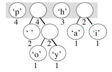
Note when we build a combined node, it doesn't represent a character like the leaf nodes do. These *interior nodes* are used along the paths that eventually lead to valid encodings, but the prefix itself does not encode a character.
