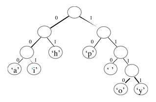
The path to 'h' is just left right or **01**, the path to 'y' is right-right-right or **1111**. Notice that the prefix property of the Huffman encoding is visually represented by the fact that characters only occupy leaf nodes (i.e. those nodes which are not a prefix of any further nodes).
