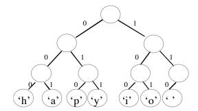
In the above tree, the encoding for 'y' can be determined by tracing the path from the root to the 'y' node. Going left then right again represents a **011** encoding.
