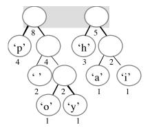
And finally, we combine the last two to get our final tree. The root node of the final tree will always have a weight equal to the number of characters in the input file.
