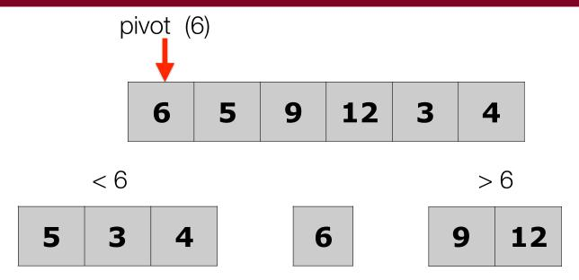
Partition into two new lists -- less than the pivot on the left, and greater than the pivot on the right. Even if all elements go into one list, that was just a poor partition.
