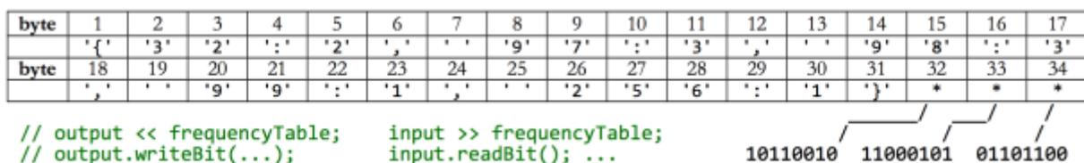
Looking at this new rendition of the compressed file, you may be thinking, "The file isn't compressed at all; it actually got larger than it was before! It went up from 9 bytes ("`ab ab cab`") to 34!" That's true for this contrived example. But for a larger file, the cost of the header is not so bad relative to the overall file size. There are more compact ways of storing the header,
