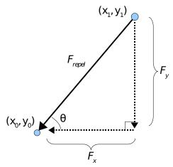
Here,  $F_x$  and  $F_y$  are the forces in the x and y directions exerted on the node  $(x_0, y_0)$ . Using some simple trigonometry, we get that
