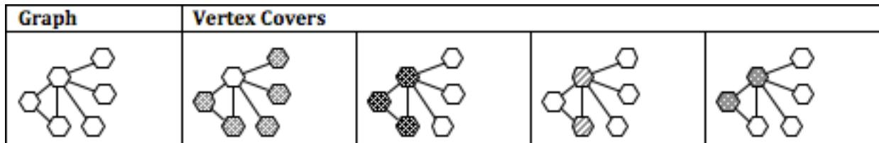
Each of the four illustrations after it on the right shows some vertex cover (shaded nodes are included in the vertex cover, and hollow ones are excluded). Each one is a vertex cover because each edge touches at least one vertex in the cover. The two vertex covers on the right are *minimum* vertex covers, because there is no smaller vertex cover.
