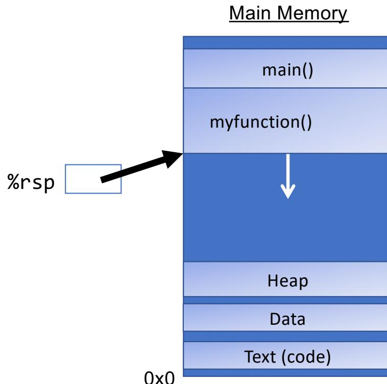
**Key idea:** **%rsp** must point to the same place before a function is called and after that function returns, since stack frames go away when a function finishes.
