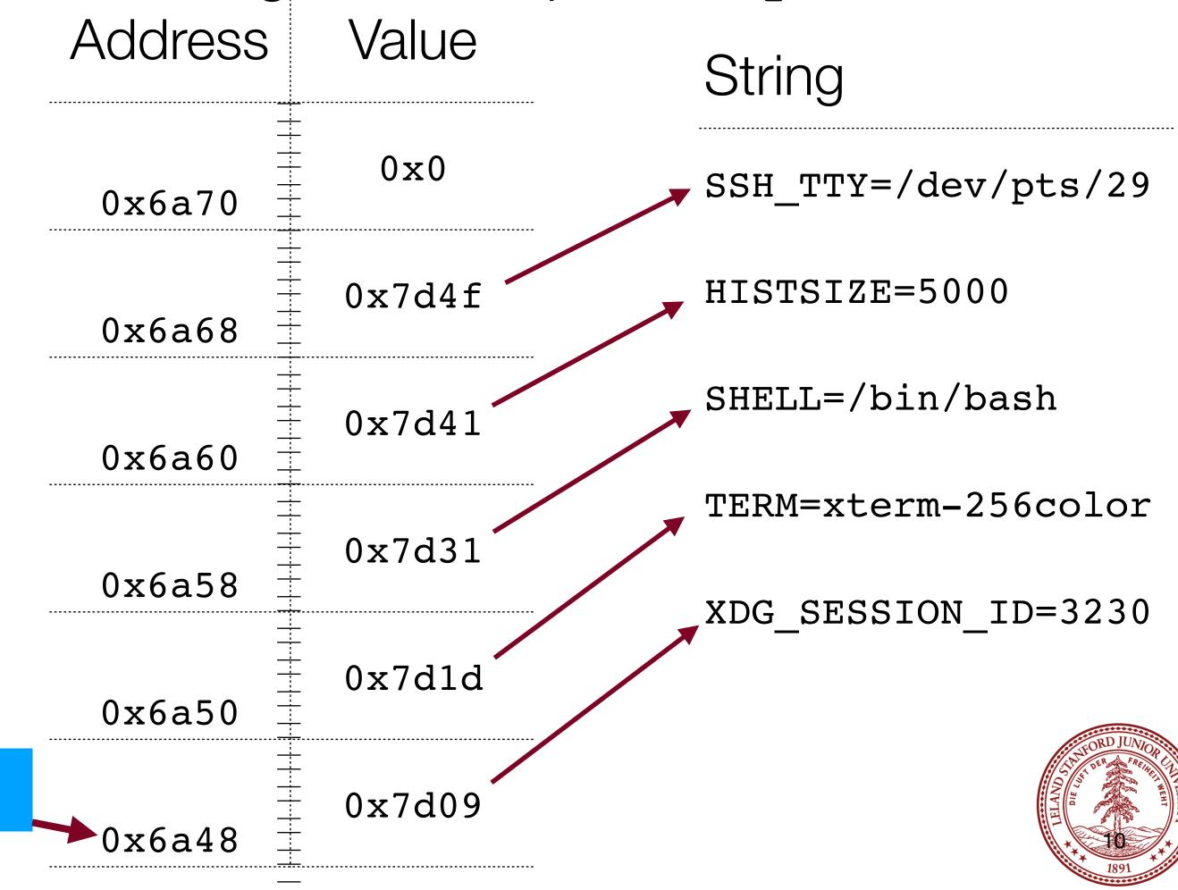
One tricky part of CS 107 for many students is getting comfortable with what the memory looks like for pointers to arrays, particularly when the arrays themselves are filled with pointers. This week's assignment has a good example: envp.
