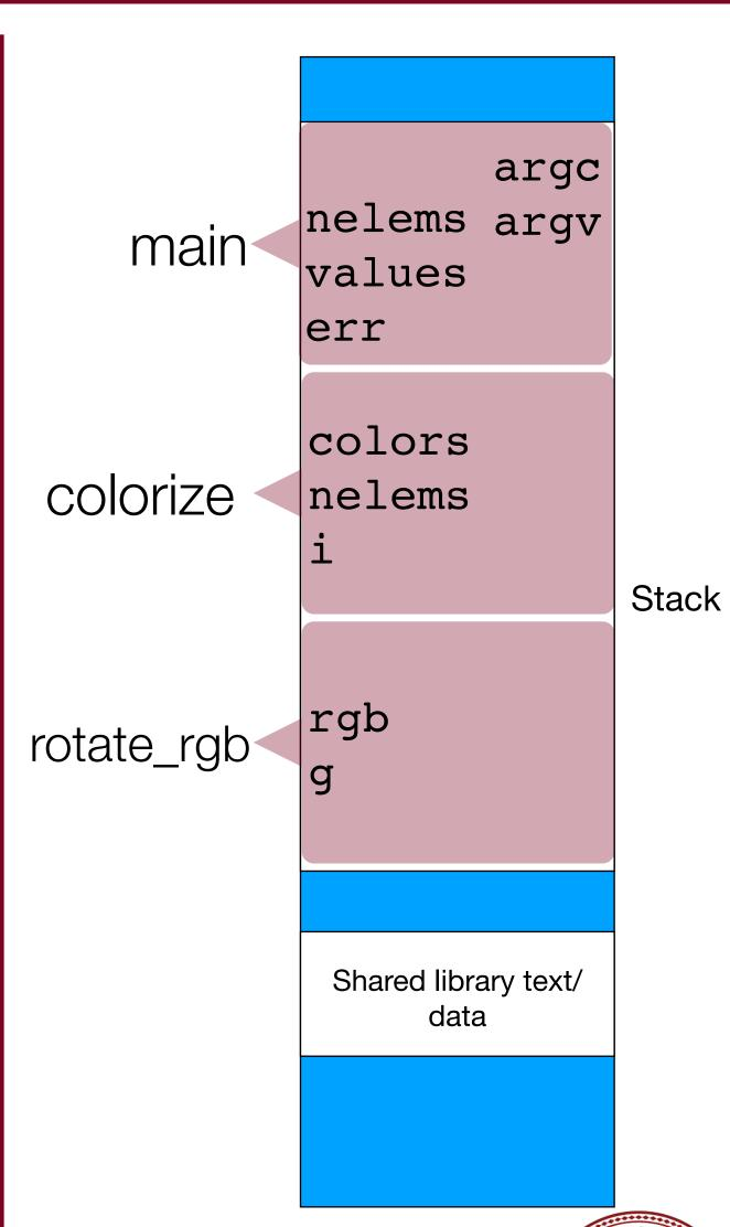
Every time you call a function, the data for the current function needs to be saved. The x86 operating system handles this in an elegant manner: a function just uses memory farther down in the stack, and leaves the part of the stack that the calling function was using unchanged. Example:
