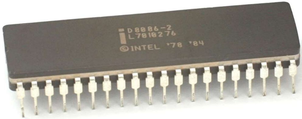
Intel 8086, 16-bit microprocessor ($86.65, 1978)
