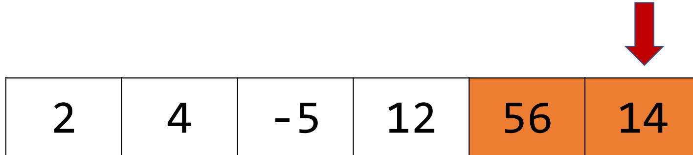
Bubble sort repeatedly goes through the array, swapping any pairs of elements that are out of order. When there are no more swaps needed, the array is sorted!
