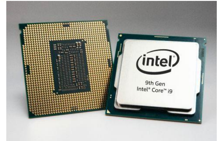
Intel Core i9-9900K 64-bit 8-core multi-core processor ($449, 2018)
