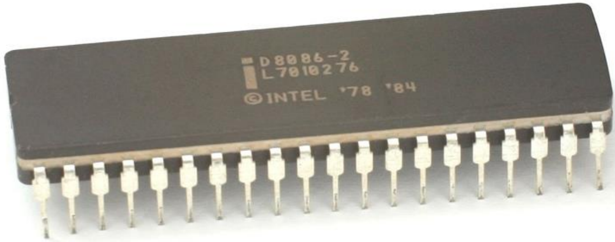
Intel 8086, 16-bit microprocessor ($86.65, 1978)
