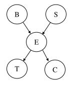
Using our background knowledge, we decide to focus on trajectory deviation (T) and communication loss (C). We know that both of these issues are a result of electric system failure (E), which can result from either battery failure (B) or solar panel failure (S). For each variable, let 1 correspond to the failure occurring, and 0 otherwise.
