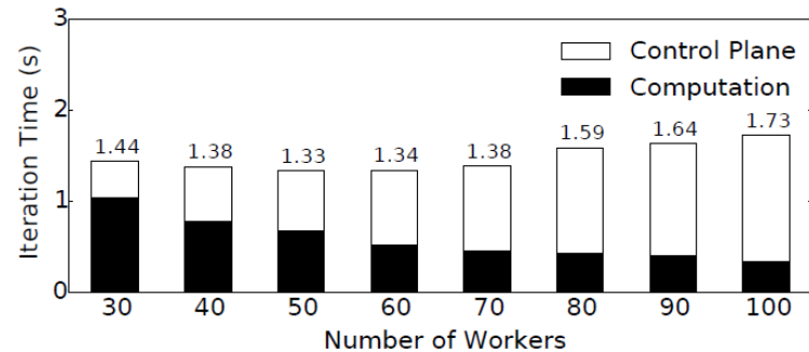
Figure 1: The control plane is a bottleneck in modern analytics workloads. Increasingly parallelizing logistic regression on 100GB of data with Spark 2.0's MLlib reduces computation time (black bars) but control overhead outstrip these gains, increasing completion time.
