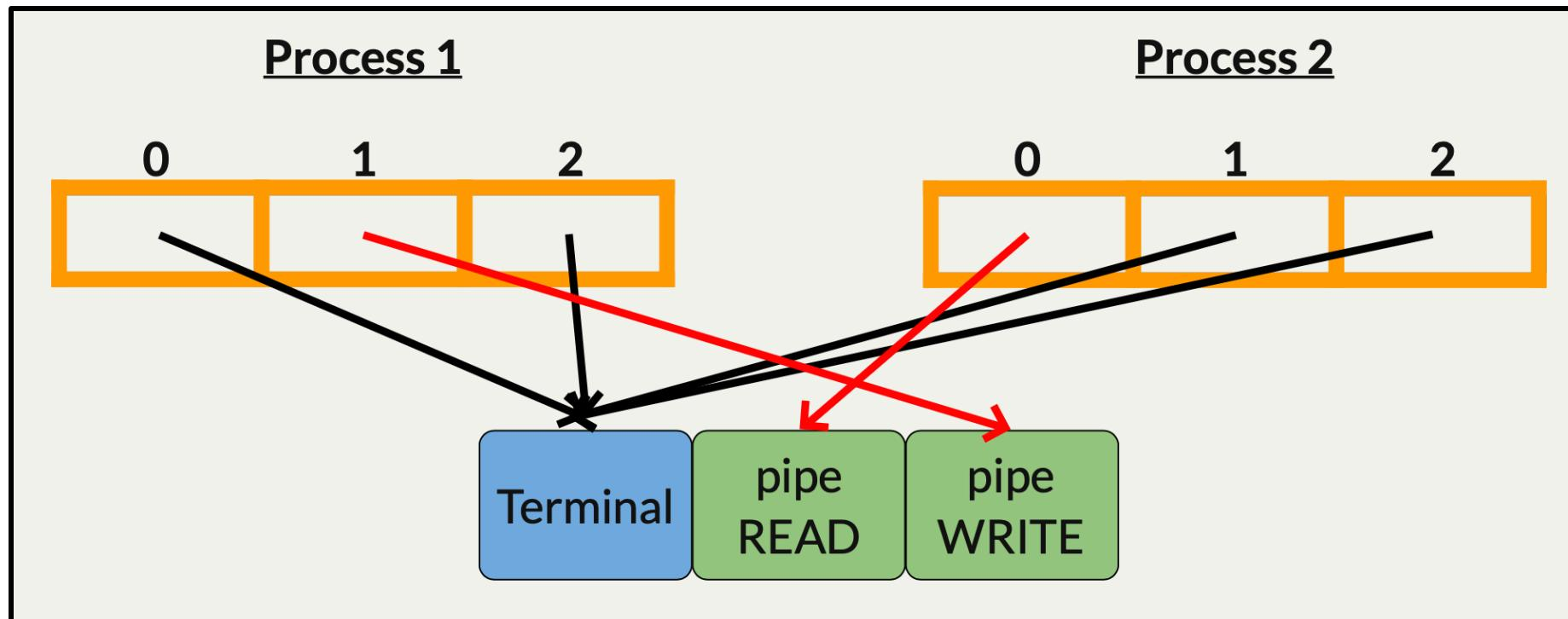
This is how piping works in the terminal! And the executables don't know they are using a pipe.
