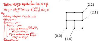
where we have only drawn the roads that are not blocked. You want to count the number of ways to get from (0,0) to (n-1,n-1), using paths that only go up and to the right. In the example above, the number of paths is 3.
