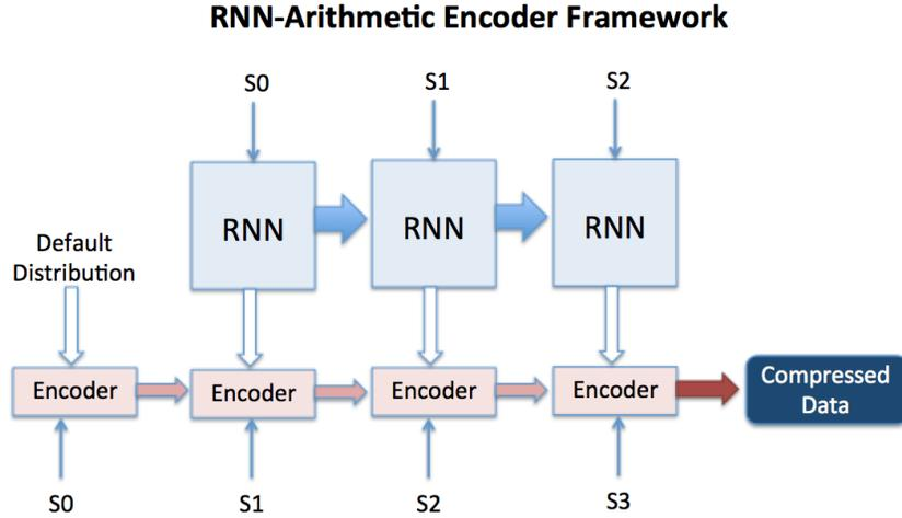
Figure 3: Encoder Model Framework
