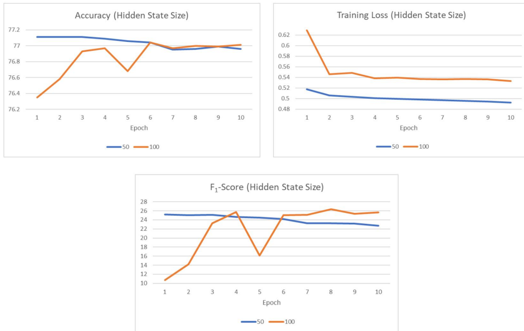
Figure 9: The accuracy, training loss, and F_1 -score of models with different hidden state sizes in the ten training epochs. The accuracy and F_1 -score were calculated on a validation data set; the training loss was calculated on a training data set. The hidden state size of 100 performed better.
