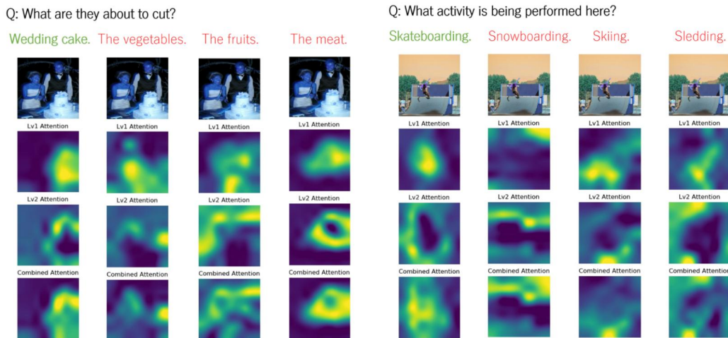
Figure 6: Spatial attention represented as heatmap. The first row are the original images, the second row are heatmaps for attention from the first attention layer, the third row are heatmaps from the second attention layer, and the last row are heatmaps for the combined attention (i.e. sum of first and second layer).
