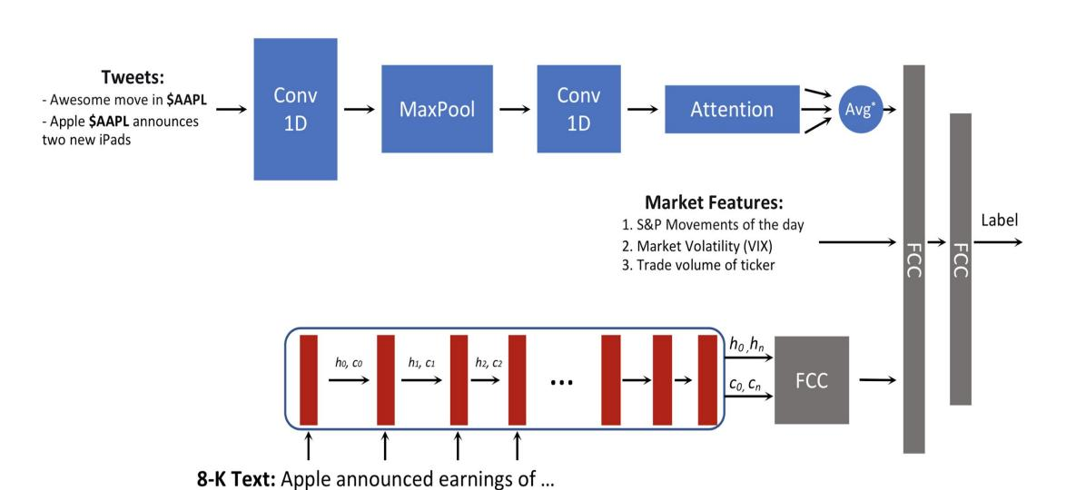
**Fig 1.** Main model used for task 2. For each data point we send a stack of 100 tweets through the CNN and then we compute an attention distribution over all the tweets passed in.
