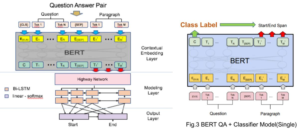
Fig.2 BERT QA Model with Modified Output layer
