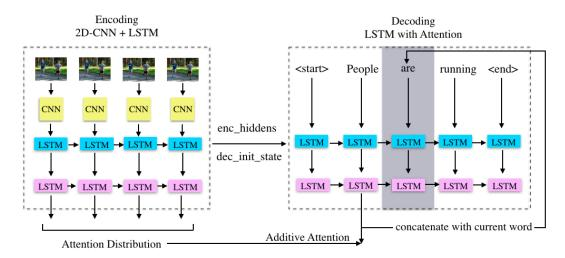
Figure 1: 2D-CNN-LSTM Encoder with LSTM Decoder: Training time architecture.
