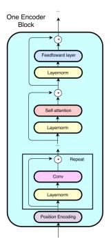
Figure 1: A visual representation of an Encoder Block, consisting of convolutional layers and multi-head self-attention.
