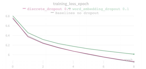
Figure 1: Training loss curves for Transformer-XL models. Grey is the baseline model without dropout. Green is the word embedding dropout model. Pink is the discrete embedding dropout variation.
