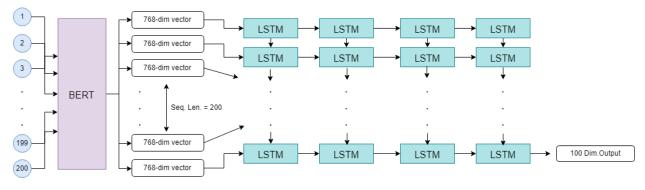
Figure 2: LSTM architecture
