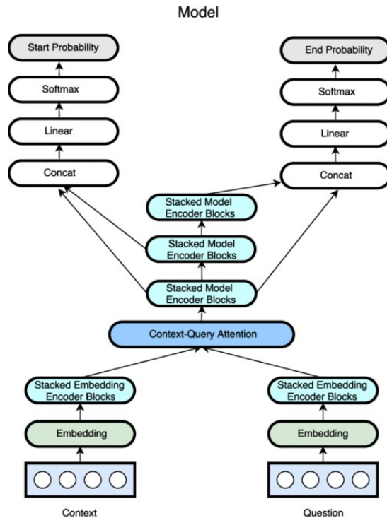
Figure 2: QANet model architecture [7]. Each input (context and query) are embedded, encoded, and then mixed via an attention layer. The resulting representation is then encoded several more times, before final neural networks are applied to predict the start and end positions of the answer.
