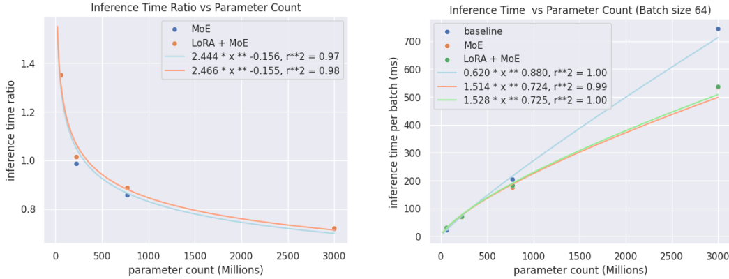
(a) Ratio of inference time of MoE'd models as a function of model size. Note that both MoE models and MoE + LoRA models are well approximated by O(\text{size}^{-0.15}) .
