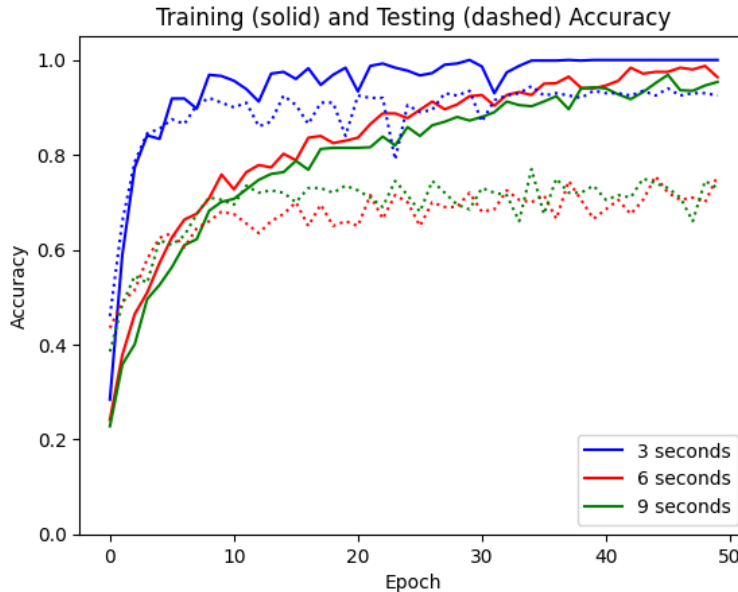
Figure 1: Training accuracy (solid) and testing accuracy (dashed) of the GTZAN data on the LSTM model
