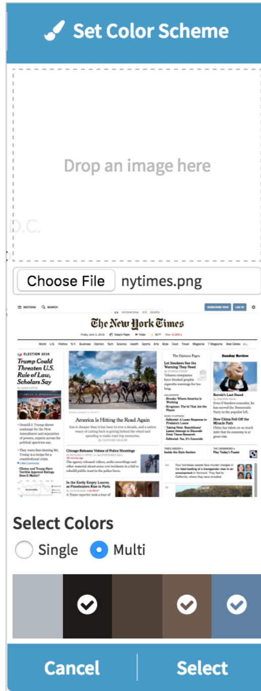
Figure 2: The image color extraction system. After the user uploads an image, the primary colors are extracted and the user can select which colors to use in their chart.
