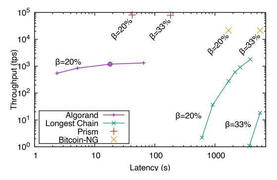
Figure 1: Plot of throughput versus latency for several protocols.
