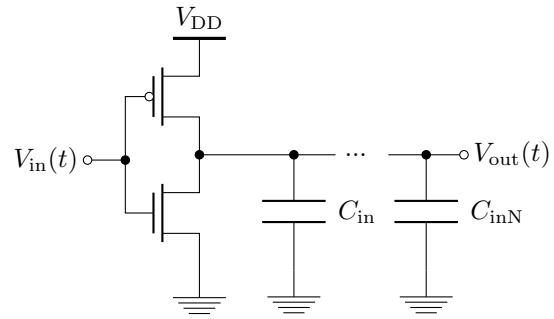
(b) Assuming that connecting an inverter to the output of an inverter is equivalent to connecting a  $50\text{ fF}$  capacitor ( $C_{in}$  in the figure above). How many inverters can be connected to the output of an inverter if the output voltage should reach  $4.5\text{ V}$  or  $0.5\text{ V}$  by half the 'on' time to be read as a valid 1 or 0?
