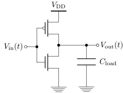
(a) Plot  $V_{\text{out}}(t)$  given that  $V_{\text{in}}(t)$  is a square wave that transitions between 0 and 5 V with a period of 50 ps. You are also given that  $C_{\text{load}} = 100 \text{ fF}$ .
