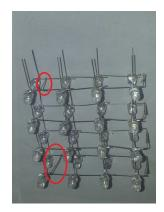
Repeat these steps to create another 2-plane module of the third and bottom plane. Bend the bottom's anode (+) leads up toward the LEDs, and the third planes leads down. After you complete this step, you will have two half cubes. Now all you need to do is to solder them together.
