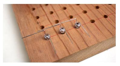
After placing all the LEDs in a row, you can solder the anode (+) terminals that are running horizontally together to form the common anode (+) terminal for that row. Then you can bend and place the next row
