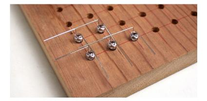
These cathode (-) leads should nicely fit under the common anode (+) terminal of the row you have already soldered. You can solder each of the anode (+) terminals of this row together to form the next common anode (+) terminal of the array, and then you need to solder the cathode (-) terminals to connect the two rows together. Continue to add rows until you complete the full array which is shown below:
