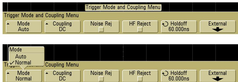
3. Press the **Edge** button in the trigger section of the oscilloscope. Then, using the menu at the bottom of the screen:
