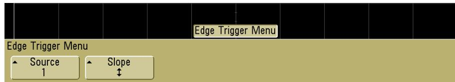
The oscilloscope will horizontally align the plot so that the **trigger event** happens at  $t = 0$ . You adjust where  $t = 0$  is on the display using the **time offset** knob (the small knob in the “Horizontal” section described above).
