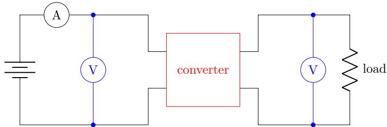
**L2:** Carry out the measurements above for each of the following resistors. Use two  $27\Omega$  resistors in parallel to get  $13.5\Omega$ .
