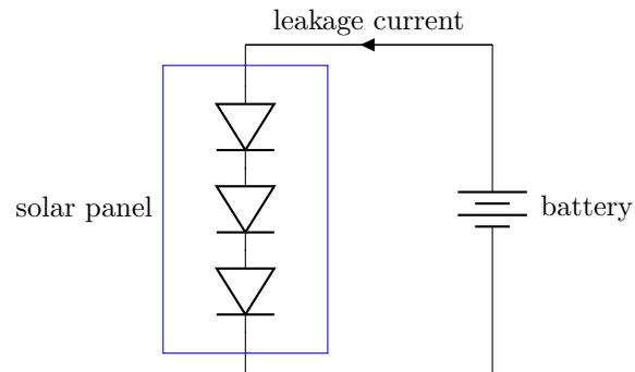
**P8:** Measure this *leakage current* by measuring the current through the cell when it is connected directly to your battery.
