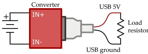
So that you can connect load resistors to the USB port, prepare a USB cable as follows: Cut the USB cable in half, and strip back the outer jacket on the USB-A (big connector) side. Strip about  $1/4"$  of the 5V and ground wires (red and black respectively), and tin the ends by melting a small bit of solder onto the wire.
