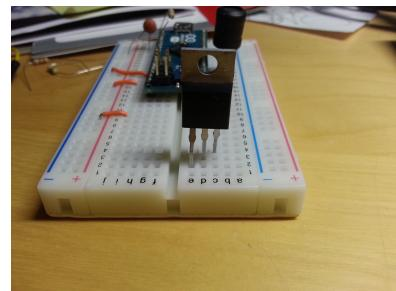
To measure the on and off resistances of the nMOS transistor, we'll want to connect the source to ground, so that we can control the gate-source voltage. The gate connects to 5V, GND or nothing (floating), depending on the measurement. Do **not** connect the drain to anything other than the ohmmeter.
