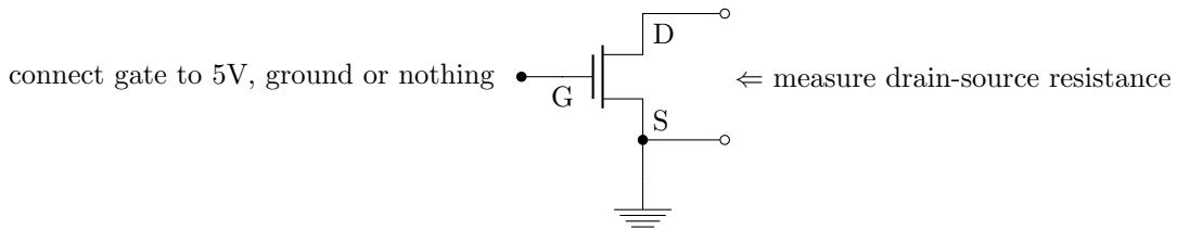
**Important measurement technique:** All wires have some resistance, including the leads of your multimeter. This means that even when you touch the two probes together, you won't measure zero resistance. Since this is typically less than  $1\Omega$ , it can usually be ignored. But if you are measuring a small resistance, you should measure this baseline resistance first, and subtract it from the resistance you measure.
