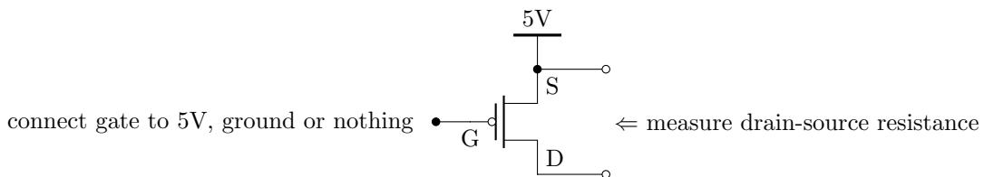
**P7:** What is the drain-source resistance of the pMOS transistor when the gate is (a) connected to 5V, (b) floating and (c) connected to GND?
