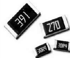
Figure 2.4: Resistors come in many different shapes and sizes. The resistors on the lower right are surface mount resistors.
