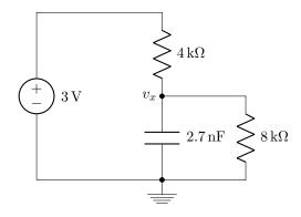
**Example 7.** The circuit below has reached steady state.
