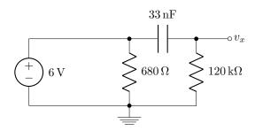
**Example 8.** The circuit below has reached steady state. What is the voltage  $v_x$ ?
