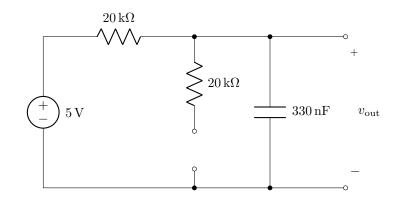
Since  $v_{in}(t) = 0$  for all t < 10 ms, the circuit is in steady state at  $t = 10 \text{ ms}^-$ . Furthermore, that  $20 \text{ k}\Omega$  resistor on the right doesn't do anything while the transistor is off. So the circuit reduces to this:
