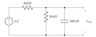
The voltage  $v_{\text{out}}$  is the voltage across a capacitor, which can't change instantaneously, so  $v_{\text{out}}(10 \text{ ms}^+) = v_{\text{out}}(10 \text{ ms}^-) = 5 \text{ V}$ . (Caution! The logic isn't that the *output voltage* can't change instantaneously, it's the the voltage across the capacitor can't.)
