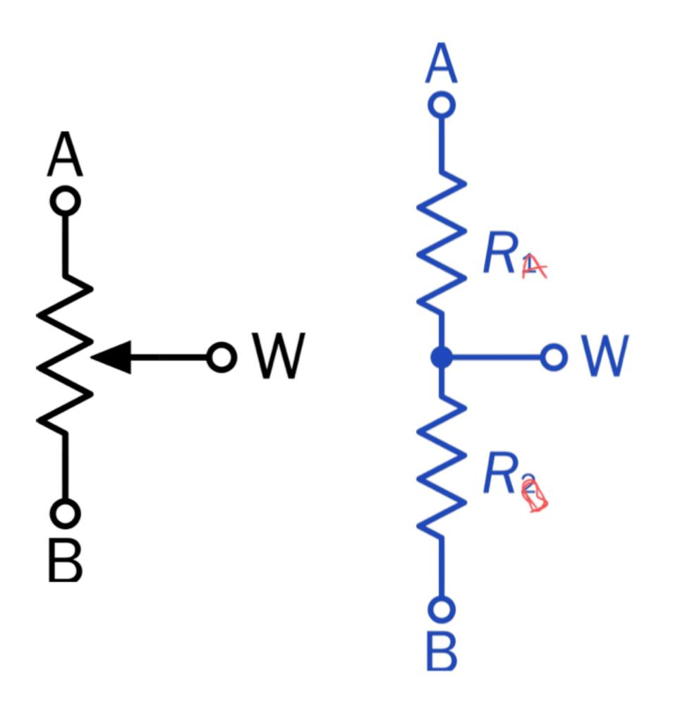
$R_1$  and  $R_2$  vary with the wiper, but  $R_1 + R_2 = \text{constant}$
